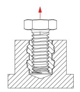
**Pullout** is the force required to pull the insert from the sheet.
